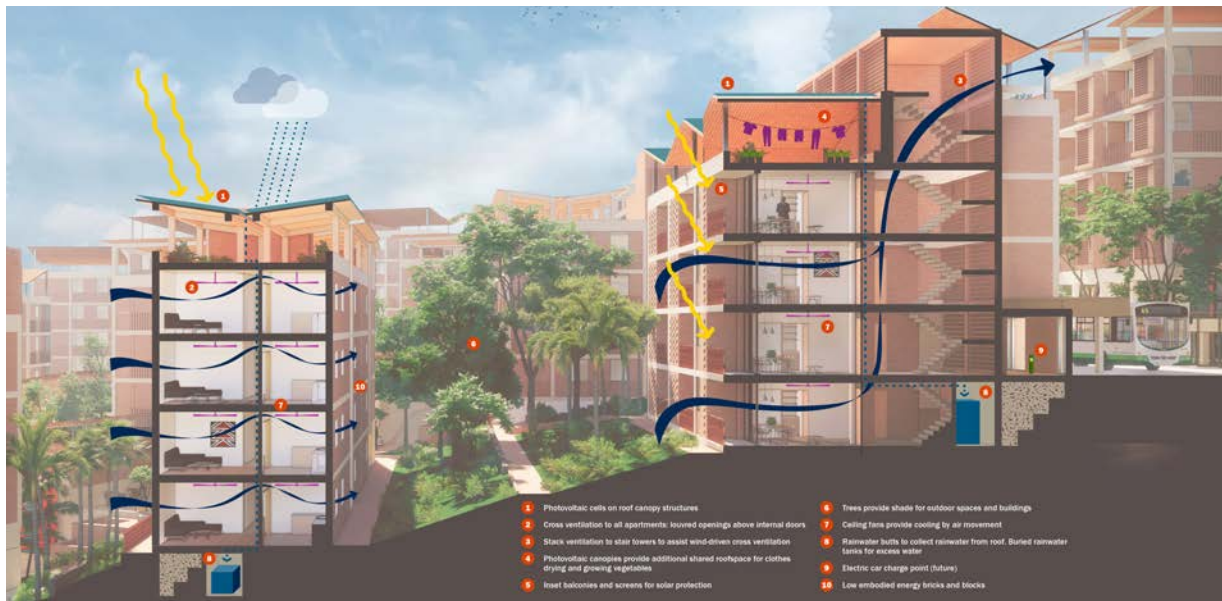
Figure 44: Sustainable solutions integrated at building and street level (src: confidential)
